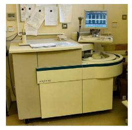
antibody and labeled digoxin, and if there's digoxin in the serum, it will compete with the labeled drug for the antibody, and that means some fluorescent digoxins *won't* be bound by antibody, and there will be less polarized fluorescence emitted. Long to say but quick to do: in a big lab, these are done by large mysterious machines fueled by reagents supplied by the machine manufacturers, and fed robotically with test samples.
